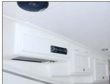
Moulded fibreglass overhead cupboards with gloss white doors.
