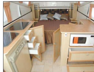
The standard configuration includes five drawers, two robes, five cupboards, eight overhead cupboards, two drop down flaps and a storage locker behind the seat.
